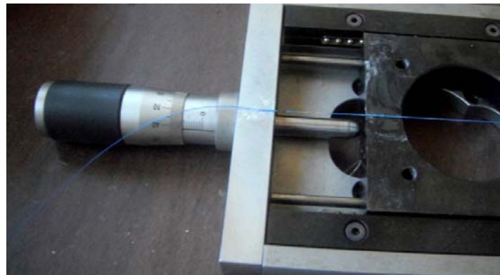
Figure 3. Detail of the stretching setup for FBG1. The fiber is glued at the stage frame and at the moving block, 10 cm apart, with super glue allowing the stretching of FBG1 that is positioned between these points.
