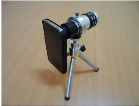
Fig. 2. Picture of a smart-phone with an 8× telescope accessory.
