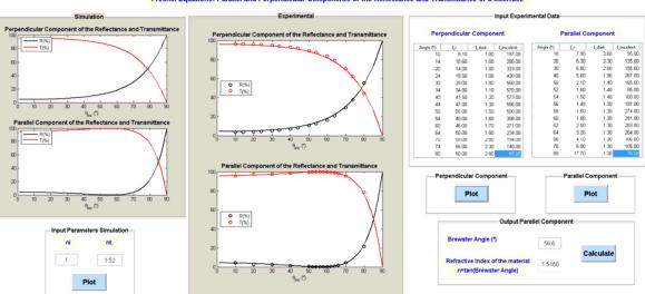
resnel Equations: Parallel and Perpendicular Components of the Reflectance and Transmitance of a interface
