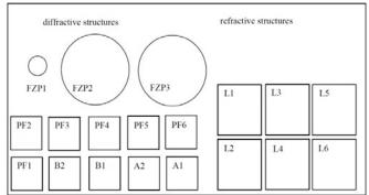
Figure 1. Distribution of the different microoptic elements on the plastic card
