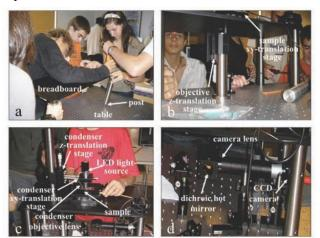
FIG. 2: Construction of the microscope: (a) the microscope platform; (b) the sample xy-translation stage; (c) illumination LED and condenser lens; (d) imaging.
