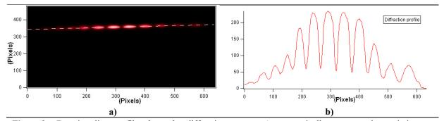
Figure.2: Drawing line profile along the diffraction pattern a) automatically generate the variation intensity b).
