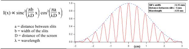
**Figure.3**: Plots of the expression of I(x). The dashed line corresponds to the squared sinus cardinal and the solid line to the squared cosine function.
