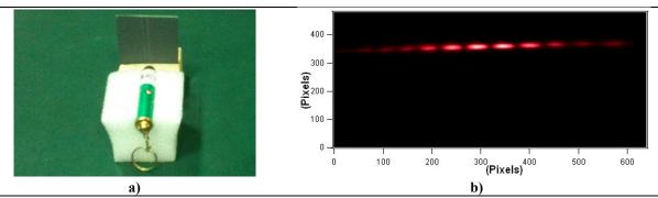
**Figure.1**: a) Laser pointer fixed on a small patch of polystyrene ahead slits made by cutter on a backside of mirror. b) Diffraction-interference pattern figure observed at 5 m from the mirror with a 635nm wavelength.
