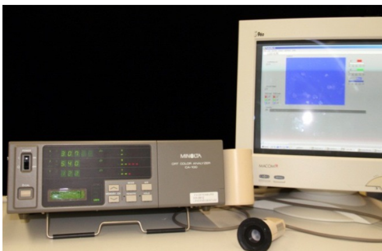
Figure 6. The testing environment of the Konica Minolta CRT Color Analyzer CA-100
