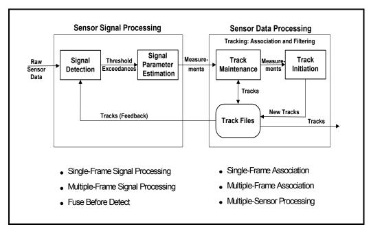
Figure 1. Sensor Signal and Data Processing
