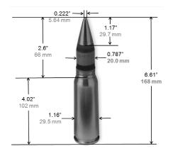
Figure 2. Typical munitions/dimensions for a popular M940 Bullet
