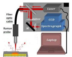
Figure 7. Fiber optic spectroscopy method for obtaining Raman spectrum results for propellant stabilizer (i.e., MNA)
