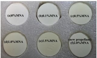
Figure 8. Photo of laboratory samples that have (a) 100% Aluminum Oxide  $(Al_2O_3)$ , (b)  $Al_2O_3 \& 0.1 \%$  MNA, (c)  $Al_2O_3 \& 0.5 \%$  MNA, (d)  $Al_2O_3 \& 1\%$  MNA, (e)  $Al_2O_3 \& 1.5 \%$  MNA, and (f)  $Al_2O_3 \& 2\%$  MNA
