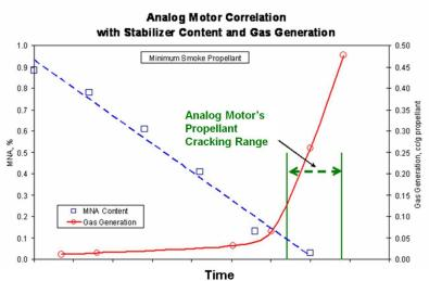
Figure 1. Stabilizer depletion (dash line) verses propellant generated off-gassing
