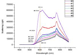
Figure 6. Measured results showing absorption spectrums for samples of un-aged propellant (sample #0) and propellant samples that experienced up to 25 years of accelerated aging
