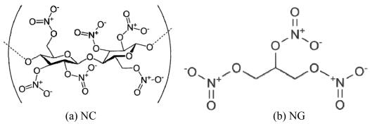
Figure 4. Molecular structures for (a) nitrocellulose and (b) nitroglycerin <sup>3,4</sup>
