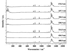
Figure 10. Measured results by Szostak et al of the Raman spectra of powdered MNA
