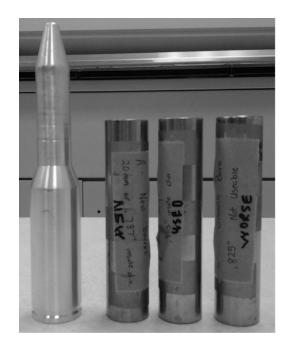
Figure 12. Mock gun barrels of approx. ~4inch length; outer diameters of all three barrels are 1.000 inch; inner diameters are 0.787 inches (simulating a new barrel), 0.805 inches (simulating a used barrel), and 0.825 inches (simulating a condemned/worse case barrel)
