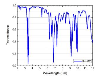
Fig. 3. Measured transmittance spectrum of IR-M2 in the IR region with cell gap  $d=21 \mu m$
