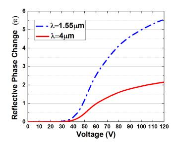
Fig. 4. The voltage-dependence phase change curves of PNLC sample in a reflective mode at  $\lambda$ =1.55µm and  $\lambda$ =4µm, respectively
