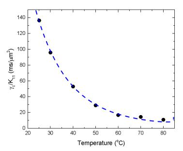
Fig. 2. Temperature dependent visco-elastic coefficients of IR-M2: black dots are measured data and blue dash line is fitting with Eq. (2) at  $\lambda$ =633nm.
