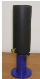
Fig. 8. Cylinder reservoir with illuminators.
