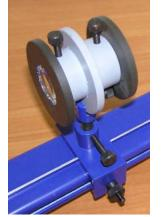
Fig. 7. Light beam expander (collimator).
