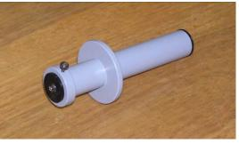
Fig. 6. Horizontal projecting microscope.
