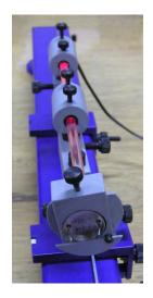
Fig. 16. Studying the loss caused by air gap between elements.
