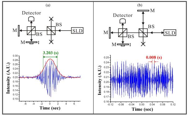
Fig. 5. Experimental setups (top) and measured interference patterns (bottom) for (a) the case without optical feedback at a constant scan speed of 4.46  $\mu$ m/s, and for (b) another case with maximum optical feedback at a constant scan speed of 53.2  $\mu$ m/s.
