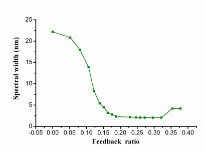
Fig. 3. The spectral width (FWHM) versus the feedback ratio curve.
