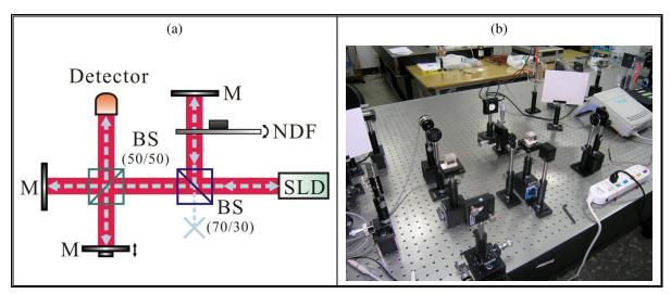
Fig. 4. (a) The schematic diagram of the experimental setup for observing the degree of temporal coherence. BS (70/30), beam splitter with the ratio of separating light of reflection and transmission at 70:30. BS (50/50), beam splitter with the ratio of separating light at 50:50. NDF, neutral density filter. M, mirror. (b) The photograph of the experimental setup.
