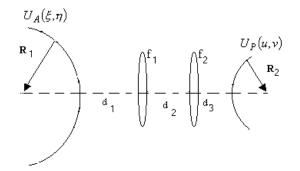
Fig. 1. Optical system between spherical emitter and spherical receiver.
