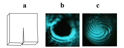
Fig. 4 Images related to the phase plate. Frame (a) shows a sketch of the wedged phase plate. Frame (b) shows a laser beam profile after passing the phase plate. Frame (c) shows an interference pattern of the beam in (b) with a portion of the beam that did not go through the phase plate.
