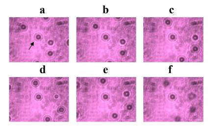
Fig. 3 Images of objects in an optical tweezer showing transverse (frames a-c) and longitudinal trapping (frames d-f). The object singled out by the arrow is the trapped 5-µm sphere.
