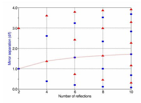
Fig. 4. This plot shows the locations of all images predicted by matrix analysis as a function of the mirror separation d in units of the focal length f. The number of images is equal to the number of reflections, and the predicted images are either inverted (squares) or not (triangles). The dashed line shows the primary image and the observed sequence of secondary images.
