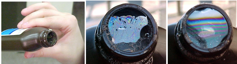
Fig. 7. Interference patterns of reflected light in soap films. Note the ‘black’ film at the top, and the white area and horizontal colored bands in the right-most picture.
