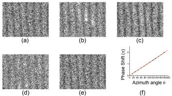
Fig.2. Interference pattern recorded onto CCD for (a)  $\theta = 0^{\circ}$ , (b)  $\theta = 45^{\circ}$ , (c)  $\theta = 90^{\circ}$ , (d)  $\theta = 135^{\circ}$ , (e)  $\theta = 180^{\circ}$ . (b) variation of phase shift as a function of azimuth of output polarizer.
