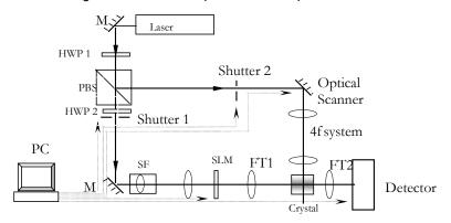
Fig.1 A schematic diagram of the experimental setup. M: mirror, HWP: half-wave plate, PBS: polarization beam splitter, SF: spatial filter, SLM: spatial light modulator, FT: Fourier transform lens, Detector: image detector array (CCD) or power meter, PC: computer. Solid lines indicate light beams, and dashed lines indicate remote control through computer interfaces.
