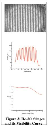
cm. The HeNe has good spatial coherence across the beam diameter. The reduction in central fringe visibility from its actual value of 1.0 gives an qualitative presence of ASE (Amplified Spontaneous Emission) and also the multi mode nature of the laser beam. The interferometer can be easily set up in college optics laboratory and it will help in visual understanding and the measurement of the coherence of the laser beam.
