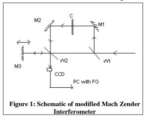
W1 and recombine at wegde W2. The one part of the laser beam propagating in the path W1 $\rightarrow$ M1 $\rightarrow$ M2 $\rightarrow$ W2 and the other beam propagating along the path W1 $\rightarrow$ W2 $\rightarrow$ M3 $\rightarrow$ W2, both the beams combine at wedge W2. C is the compensating plate. The wavefront from the earlier path is inverted along a line of folding.
