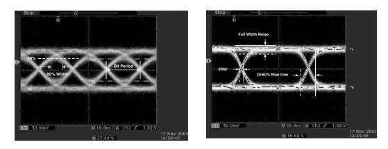
Figure 7: Sample measurements on eye diagrams.
