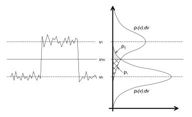
Figure 5: PDFs  $[p_i(v) dv_i, i=0,1]$  for levels of 0 and 1  $(v_0 \text{ and } v_1)$  in the presence of random (Gaussian) noise. The probabilities of error on a 0 signal  $(P_0\text{-shaded})$  and 1 signal  $(P_1\text{-hatched})$  are also indicated
