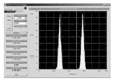
Figure 3: Q-factor analysis software showing voltage histogram and analysis results
