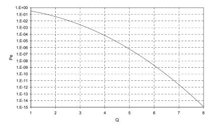
Figure 6: Error probability Pe versus error probability factor Q
