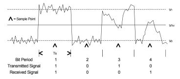
Figure 4.: Threshold detection in digital receivers, illustrating the possibility of errors in the presence of random noise
