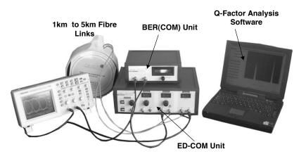
Figure 2: ED-COM and BER(COM) units in operation
