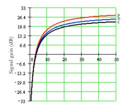
**Fig. 1.** The variation of signal gains versus launched pomp powers for the signal power regime 50  $\mu$ W. (a), (b) and (c) curves correspond to - 20 °C, 20 °C and 60 °C, respectively.  $\tau$  is taken as 10 ms and L = 15 m.
