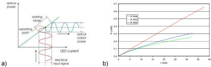
Fig.2 a) modulation of the LEDs b) PI curves of the used LEDs
