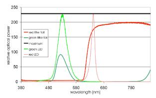
Fig.5 Absorbtion spectra of the red and green filter foil in comparison with the emitted LED power
