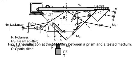
Fig. 2 Schematic diagram for measuring the two-dimensional distribution of refractive index of a material.
