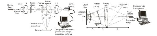
Fig.1. Experimental setups. (a) Double arm convergent correlator. (b) Imaging setup with a volume grating.
