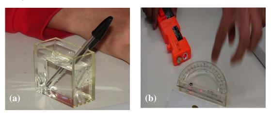
Fig. 4. Simple experiments to demonstrate (a) refraction of light and (b) total internal reflection.
