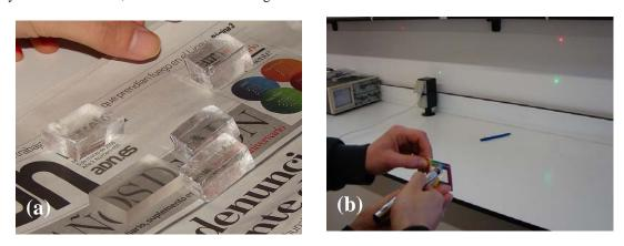
Fig. 5. Experiments to demonstrate (a) birefringence using calcite crystal and (b) diffraction from grating.
