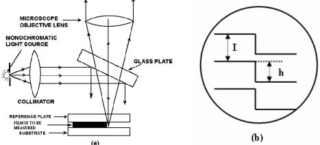
Fig. 4(a). Enlarge view of the interferometric arrangement for the measurement of film thickness; (b) The fringe pattern with step height 'h' and fringe spacing 'I'.
