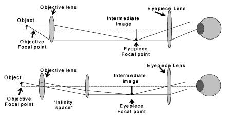
Figure 1: The basic imaging mechanisms in microscopy. Upper – the 'finite tube" configuration and lower the "infinity corrected" microscope. The latter enables non focussing optical elements to be placed in the infinity space to facilitate image enhancement.
