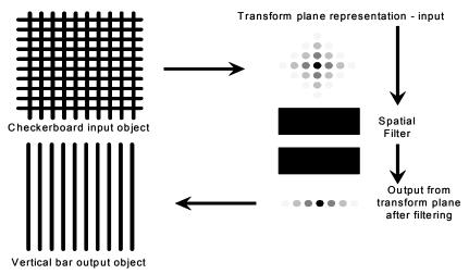
Figure 4: Illustrating the principles of spatial filtering in a 4 f system (figure 2) using a checkerboard input object and monochromatic light to highlight the diffraction pattern (Fourier transform) in the transform plane. The simple spatial filter selects one horizontal row in the transform pattern and results in the vertical bar image.
