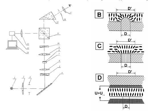
Fig.1. Optical scheme: 1-light source, 2-collector, 3-aperture, 4-mirror, 5-polarizer, 6-condenser lens, 7-object, **8-LC SLM**, 9-microscope lens, 10-analyzer, 11-prism-cube, 12-ocular 1, 13-CCD-sensor, 14-computer, 15-prism, 16-aperture, 17-ocular. B, C, D - defects types. D - real size of defect. D'- image size of defect in NLC.
