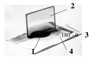
Fig.10. Mirror technique for tangent construction and contact angle  $\theta$  measurement: 1-droplet's profile; 2-reflective mirror; 3-horizontal line; 4- tangent line.
