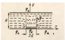
Fig.3. Solitary structural defect and local orientation of LC molecules induced by it
