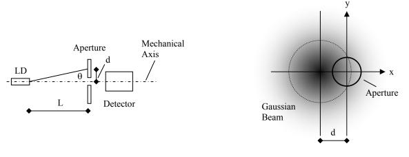
Fig. 1. Measurement setup,  $\theta$ : pointing angle.
