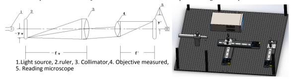
Figure 3. The principle of Tele-curriculum experiment system
