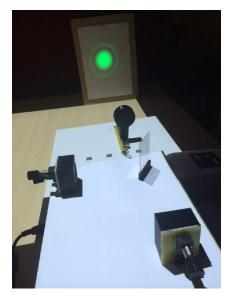
Figure 3. Photograph of the AMI setup, where the interference pattern (here rings) is projected in a surface.
