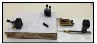
Figure 2. Replica of the Michelson interferometer.
