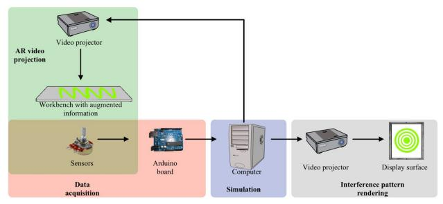
Figure 1. Flowchart describing how AMI prototype works.
