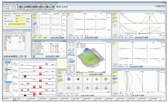
Figure 5. Some of the available diagrams showing system performance: Seidels, OPD, TRA, MTF, wavefront and more
