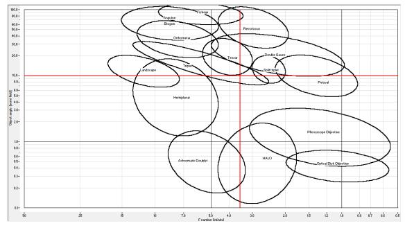
Figure 2. f/# vs. field angle for solution, showing different lens families
