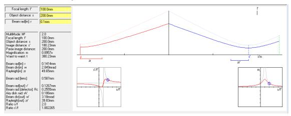
Figure 3. Laser mode: Gaussian beam profile and beam propagation factor effect
