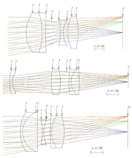
Figure 6. The three lens designs provided for the tolerance grade mapping project. (Top) Petzval lens taken from Laikin [5] and optimized in [6]. (Middle) Inverse telephoto lens taken from Laikin [5] and optimized in [6]. (Bottom) Heliar lens taken from Smith [2] and optimized in [6].
