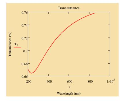
Figure 1. Calculated transmittance for a 25 nm layer of CeO<sub>2</sub> on quartz substrate.
