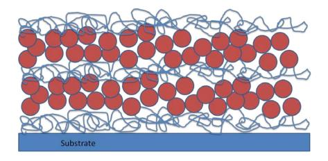
Figure 2. Schematic representation of ISAM films containing nanoparticles and polymers.
