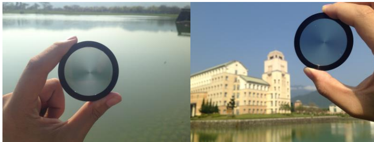
Figure 1. Axis finder is applied to observe the light polarization of lake surface reflection and blue sky from scattering.
