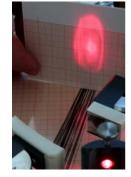
Figure 10. Beam spot at three positions in between the mirrors two and three.
