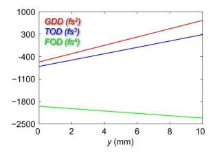
Figure 3. The dependence of the dispersion coefficients on the position of the second prism. The path length in the second prism is minimized at 0 mm and maximized at 10 mm.
