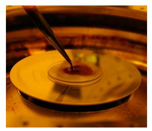
Figure 3. Lab course on microoptics: spinning of photoresist onto a substrate.
