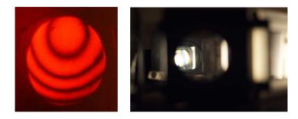
Figure 8. Left: Ring-like interference pattern obtained when illuminating the interferometer with a punctual and monochromatic (633nm) light source. **Right:** Fringes-like interference pattern obtained by illuminating the interferometer with an extended white-light source.
