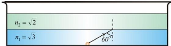
In the vessel there is some solution with refraction index  $n_1$ , above this another liquid with refraction index  $n_2$  are poured. On the bottom of the vessel there is the light source. What is the angle of the ray coming out from the vessel if the angle of incidence is 60 degrees?
