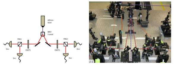
Figure 1. Experimental setup for mapping the S function with entangled photons. Red lines depict the trajectory of the entangled photons. Left: schematic. Right: photograph of the actual setup; laser is outside the picture.
