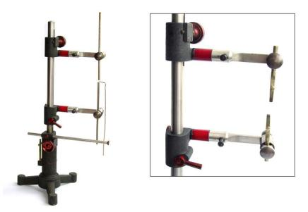
Figure 12. Gramont arc and spark stand, with metal electrodes or with spring clips (inset).
