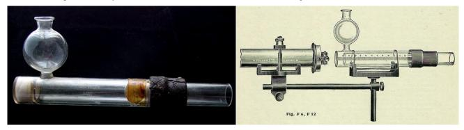
Figure 15. Adjustable absorption tube to investigate the absorption of light by liquids (Baly cell).
