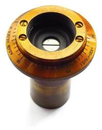
Figure 10. The symmetrical slit.
