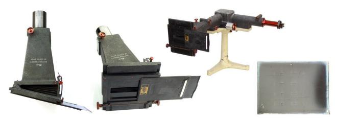
Figure 11. The photographic camera and a metal dark slide, which takes  $3\frac{1}{4} \times 4\frac{1}{4}$  inch plates (known as "quarter plates").
