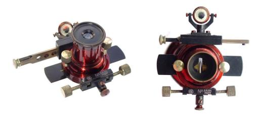
Figure 7. The shutter eyepiece.
