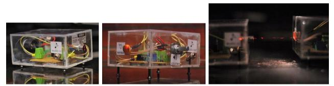
Figure 6. Pictures of our *optophonograph*. From left to right: a) transmitter, b) receiver, and c) transmitter sending signal to receiver. Signal enters the transmitter through an audio jack from any music player device, and alters the intensity of the laser. The receiver reads the laser signal with a photoresistor, and sends the electrical signal to an external speaker or earphones through an audio jack. Volume can be set in the receiver.
