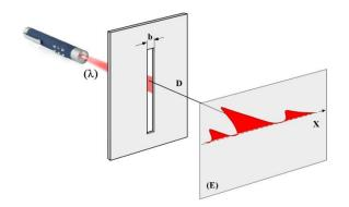
Figure 7: Diffraction obtained by a single slit with a width (d) observed on screen at a distance (D) from the slit.
