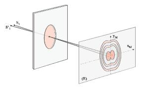
Figure 10. Diffraction by circular diaphragm of radius (r) for two sources separated by a distance d.
