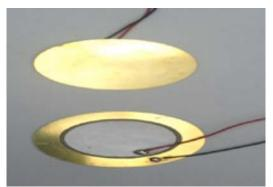
Fig. 2. Image of piezoelectric musical instrument pickups as received. Note the lightly- colored piezoelectric ceramic on one side and wire leads. The plain brass metal surface is used as the touch pad.
