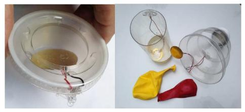
Fig. 6. (L) Shake flashlight made from a recycled condiment cup. (R) Plastic bottles cut to make drum. Here that are shown with balloons as the membrane.
