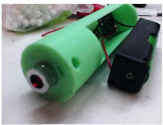
Fig. 5. The laser source mount
