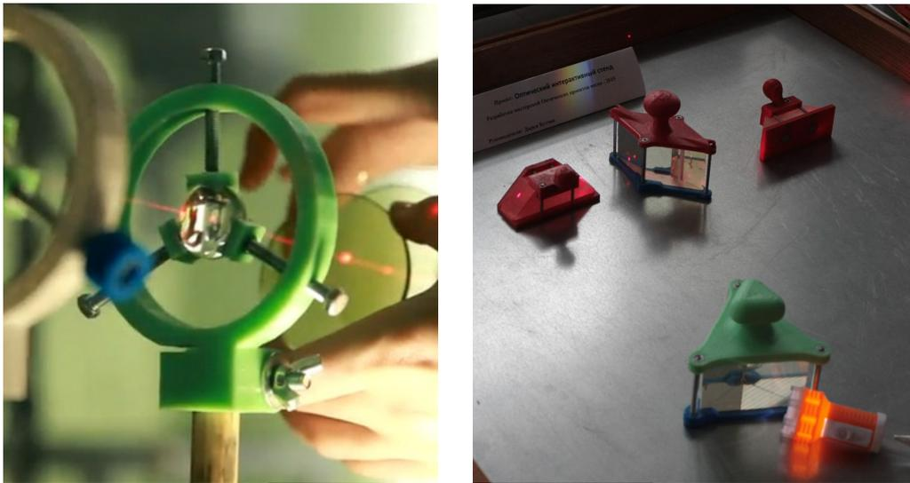
Fig. 4. The mounts for lenses and prisms
