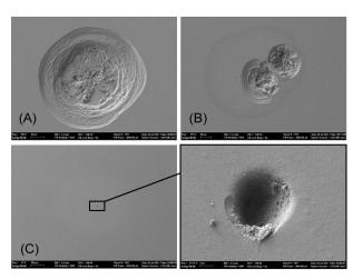
Figure 3. Typical damage morphology induced by laser irradiation with a fluence of (A) 39.2 J/cm<sup>2</sup> (p-polarized light), (B) 53.5 J/cm<sup>2</sup> (p-polarized light), and (C) 61.4 J/cm<sup>2</sup> (s-polarized light).
