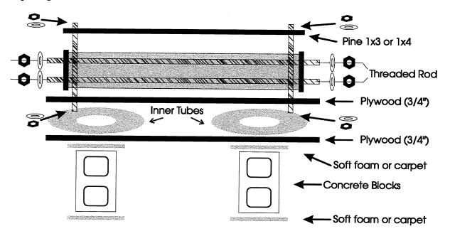
Fig. 1. Construction diagram of sand-box vibration isolation system
