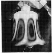
Fig. 4. Time average holographic interferogram of hand bell, visualizing one of the normal modes of vibration .
