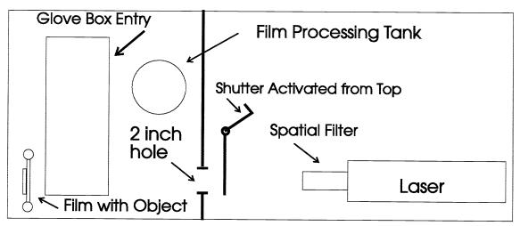
Fig. 3. Layout of demonstration reflection holography table
