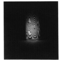
Fig. 5 Double exposure hologram of a can stressed by a rubber band. The interference pattern results from the small displacement caused by the rubber band.
