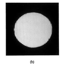
Fig. 12. Filtered spatial-frequency spectum of image (a), and resulting image showing no horizontal structure (b).
