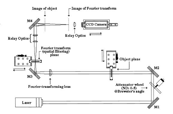
Fig. 3. System layout of "The Diffractionator".
