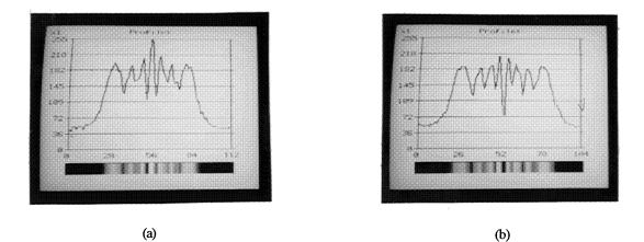
Fig. 7. Irradiance profiles across two Fresnel diffraction patterns of a circular diffracting object, first showing a central peak (a), and next showing a central minimum (b).
